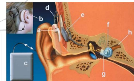
ABOVE: The Cochlear implant: (a) microphone; (b) behind the ear speech processor; (c) body worn speech processor; (d) transmitting aerial; (e) receiver stimulator; (f) electrode bundle; (g) inner ear (cochlear); (h) auditory nerve. TOP: manufactured components ready for installation.
